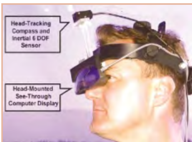
Fig 3 : Head-worn, motion-tracked displays
