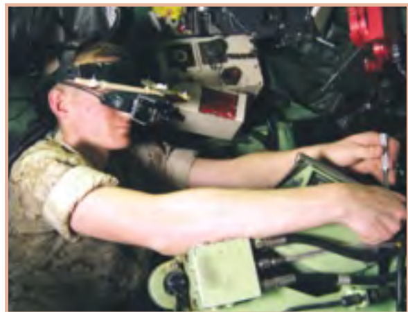
Fig 4 Tracked head-worn display to carry out maint inside an APC
